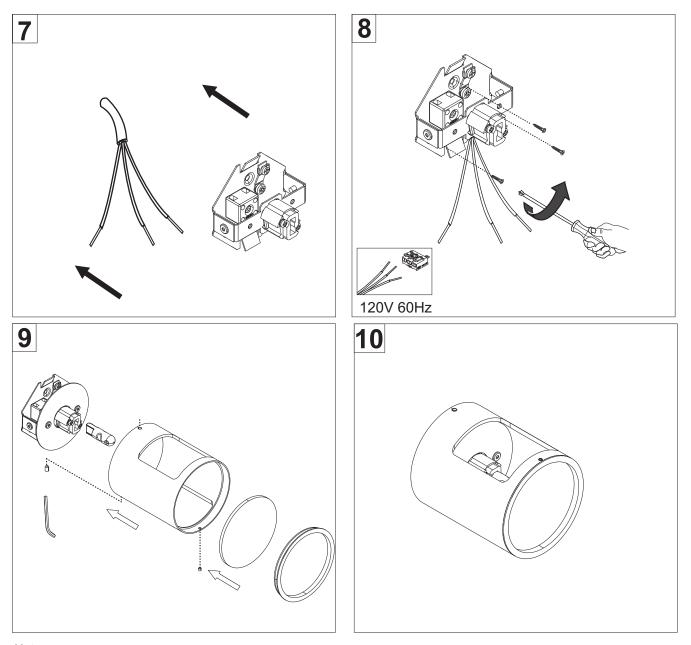
Note: Steps 7-10 is an example fixture, and are not a part of the J-Box Concealer. Mounting Piece of fixture is installed directly to wall / holes of Concealer.
